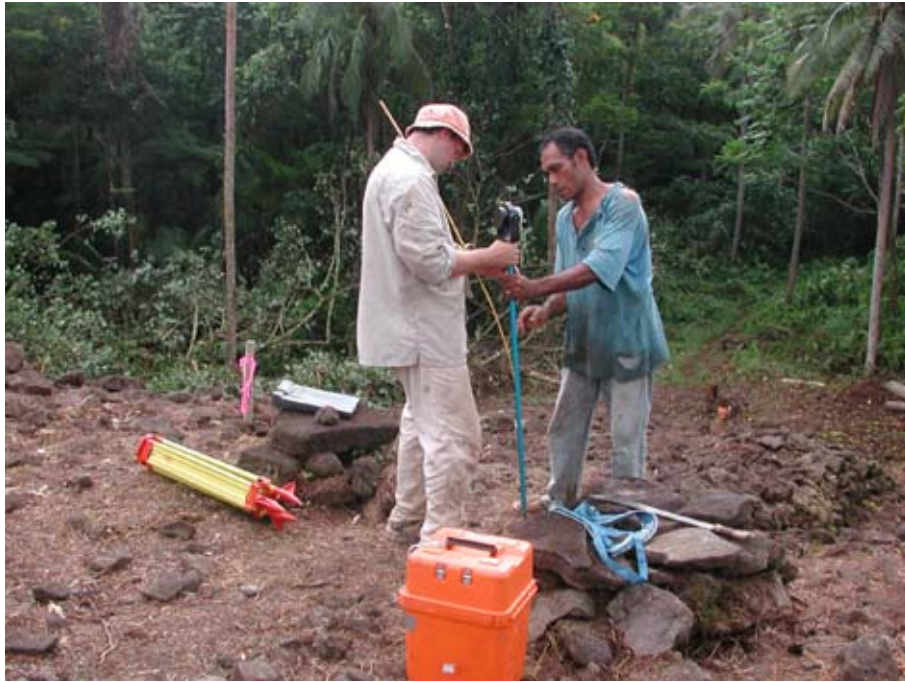
Geoff and Fito putting up the theodolite.
